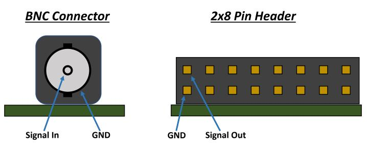
Remaining pins in the 2x8 header are not connected.
