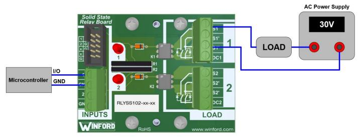
In general, the RLYSS102 is not recommended for inductive AC loads, but there are some exceptions (particularly for low AC voltages, or if there is robust inductive spike clamping in place to ensure absolute max ratings for this product are not exceeded). If there is application in which an AC inductive load needs to be controlled, please see Winford's electromechanical relay products, or contact us to discuss further.
