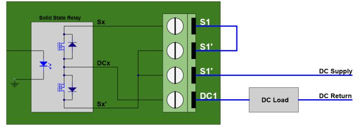
Caution: Note that if DC Supply and DC Return are swapped in the DC configuration, the load will always be powered since current will flow thru the opto-MOSFET body diodes even if the opto-MOSFETs are off.
