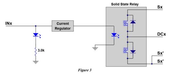
When there is sufficient current thru the LED in the solid-state relay, the opto-MOSFETs in the solid-state relay turn on, connecting Sx, DCx, and Sx'. See later sections in this document for configuration recommendations based on the type of load being controlled.
