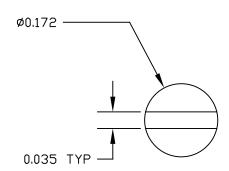
Material: Steel, Lead-free Plating: Nickel
