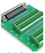
**Spring Terminals** 68 Pin Connector (BRKGDP68FV1)
