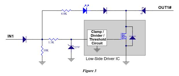
When the input is high, the low-side output FET is on (active), pulling the output down.
