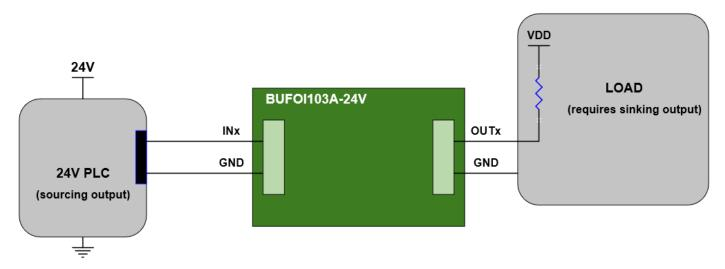
When the PLC output turns on (goes high, providing 24V signal to BUFOI103A-24V input INx), the lowside transistor that controls OUTx will turn on. This allows OUTx to sink current to ground, activating the load.
