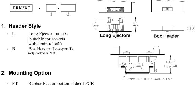
• **DIN** DIN Rail Mounting Clips
